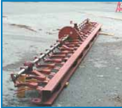
Discharge rapping system
